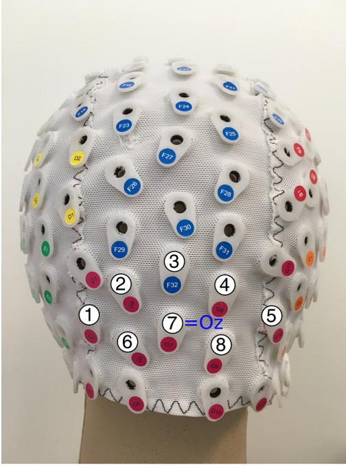
Fig. 2. Image taken by the authors of [6]. Electrode placement for the 8 EEG channels in the recordings.
