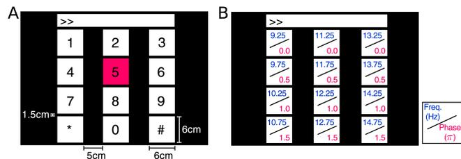
Fig. 1. Figure taken from [6]. A) Keypad display for the SSVEP-based BCI. B) Flashing frequency and phase of each button.
