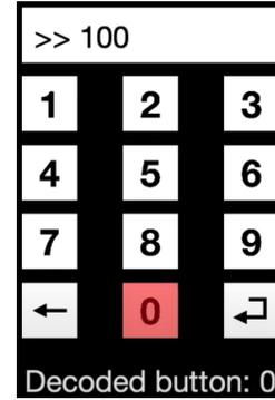
Fig. 4. Snapshot of the GUI while the simulated user is trying to type 10027. The recording data and subsequent classification just decoded a second 0.
