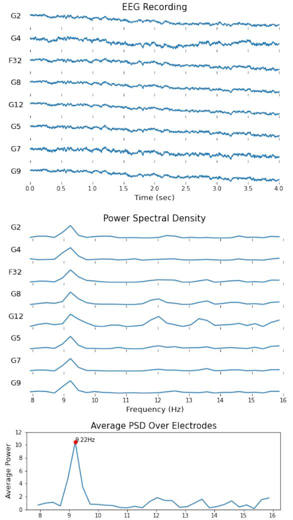
Fig. 3. Power spectral density analysis on a 4-second trial from one subject. Top) 8-channel raw EEG recordings. Middle) PSD of each electrode. Bottom) Average PSD over the electrodes and the location of the peak, which when compared to the possible button frequencies, is closest to 9.25 Hz, which is the correct decoding for this sample.
